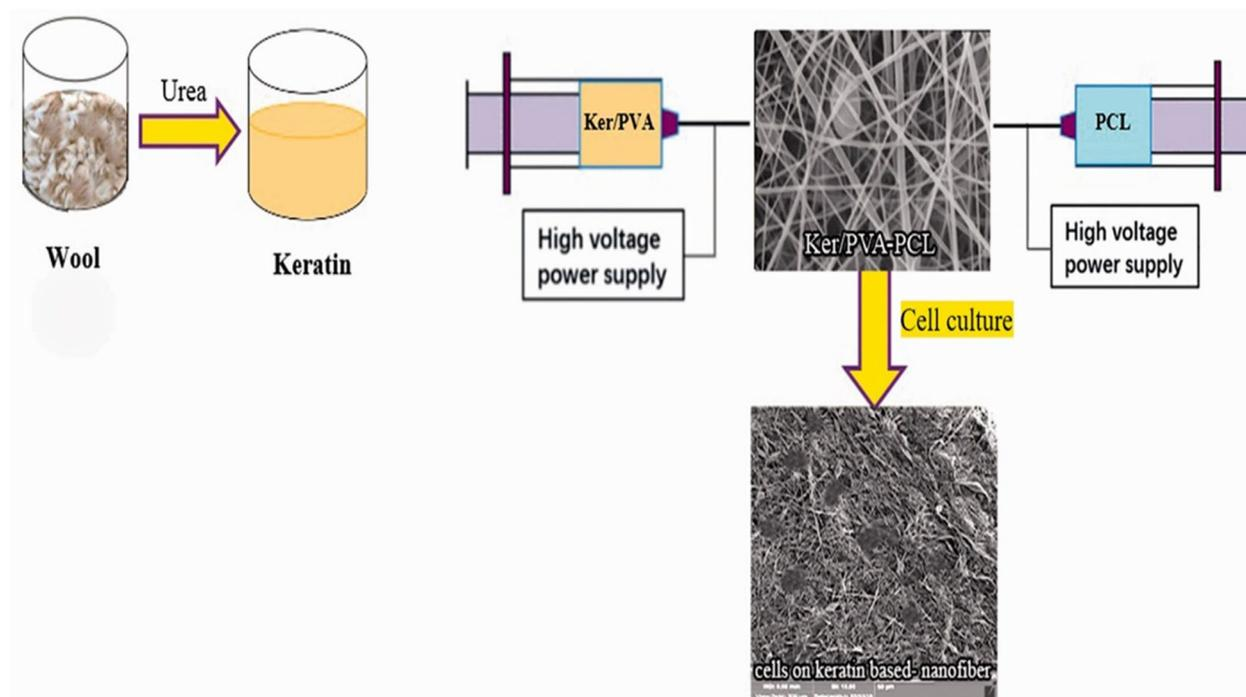
**Fig. 6** The process of making keratin-PCL Nanofiber using electrospinning technique, Reproduced with permission from reference from Ranjbar-Mohmmadi et al., 2021 [74] SAGE Journal. Open Access
